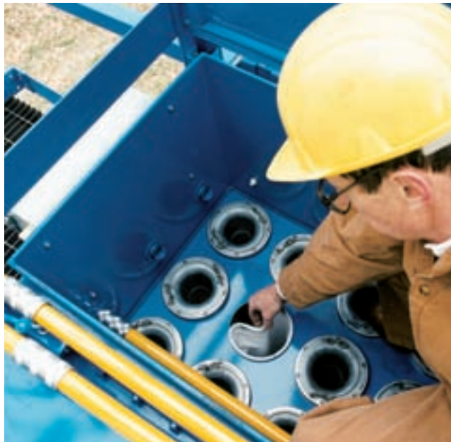
Snap ring filter bags and pulse pipes are removed and installed without tools on the STJ and CTR models.
