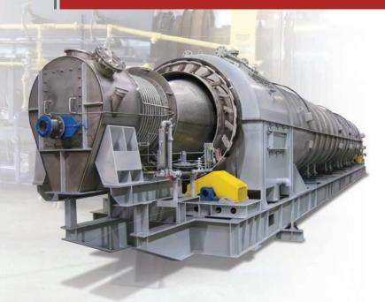
Co-current and counter-current material/ gas flow designs with multiple heating zone configurations are available. Integrated coolers provide cooling of product prior to discharge.
