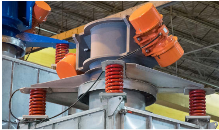
Steel Heat Shield Protects the Spiral Motors
