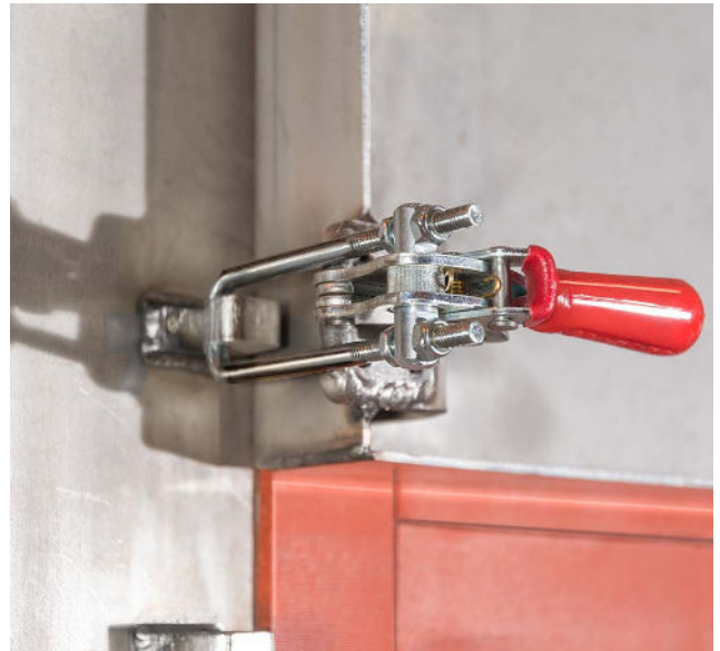
Quick Access Handles Used on Each Shroud
